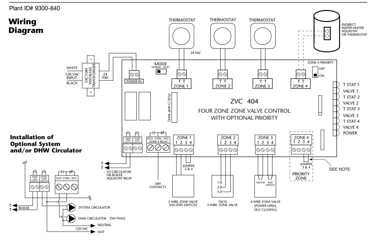
**Operation/External Diagnostics:** When any thermostat calls for heat, the appropriate zone valve is energized and the yellow light goes on. When the zone valve is fully open, the red light goes on and energizes the end switch relay. The green light should always be on, indicating that power is connected.
